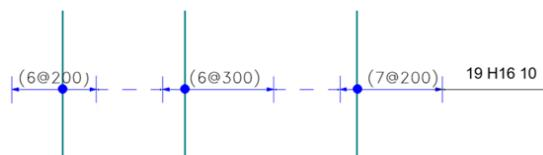
Fixed Spacing Group Annotation - showing range text for each assembly of rebar in the group.
