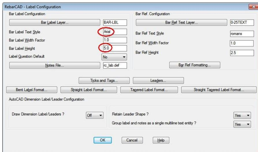
12. Type in Arial for the Bar Label Text Style and set the Bar Label Height to 5
