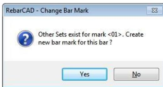
51. Answer Yes to Create a New Bar Mark for this bar. As dimension B has been edited we do not want RebarCAD to update the other sets of Bar Mark 01 to this new dimension, we need a new bar mark.
